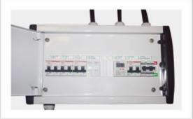
AC Prewired Box: Comes with 3 x 25A DP AC MCB, 1 x 10A DP AC MCB, 1 x Voltage Regulator, 1 x 2P AC SPD, 1 x 40A Changeover and earthing terminal. Box has cables connected on outside where you have terminals to connect your grid input and output cables.
